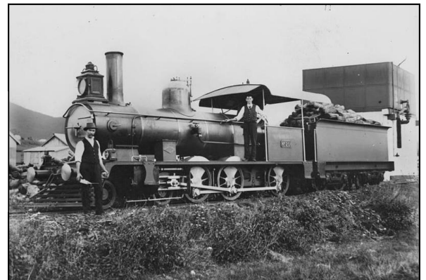
A STEAM ENGINE LOADED WITH LOGS TO BURN BEHIND IT YOU CAN SEE THE WATER TANK ON ITS STAND, AND YOU CAN MAKE OUT THE FILLING SPOUT THAT WE STILL HAVE - NOTE THERE ARE NO TREES TO BE SEEN
